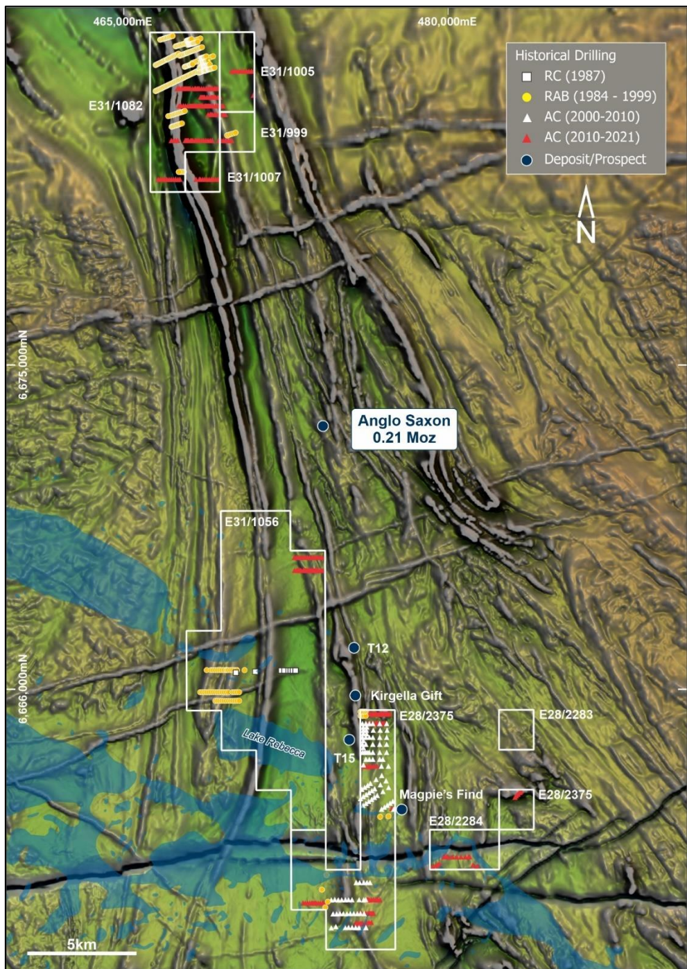
Figure 8: Pinjin JV – processed aeromagnetic data and phases / types of previous drilling shown in variously coloured shapes.
