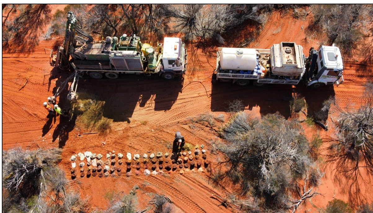
Figure 1. Image of the Aircore Drill Rig operating as part of the current drill program.
